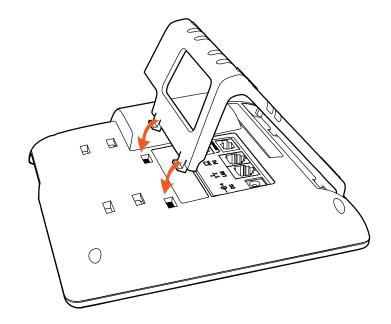
C. It is the right picture after fixing the stand bracket below:
