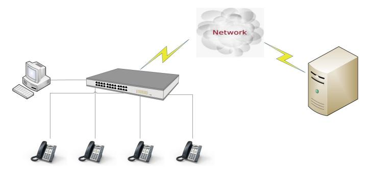
Connect LAN port to PC with Ethernet cable, or connect A10/A11/A10W/A11W to a switch/router which is in the same network as your PC. It uses DHCP mode by default, and you can review its
