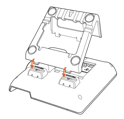
D. Press the other side joints into the slot according to the direction of the arrow
