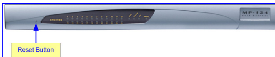
Figure 4-2: Reset Pinhole Button Location on MP-124 Front Panel
