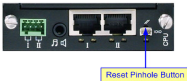
Figure 4-3: Reset Pinhole Button Location on Mediant 600 / 1000 Front Panel (CPU Module)
