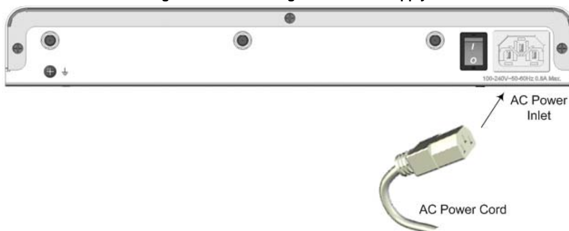
Figure 5-8: Connecting to the Power Supply
