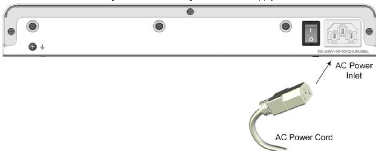
Figure 5-8: Connecting to the Power Supply
