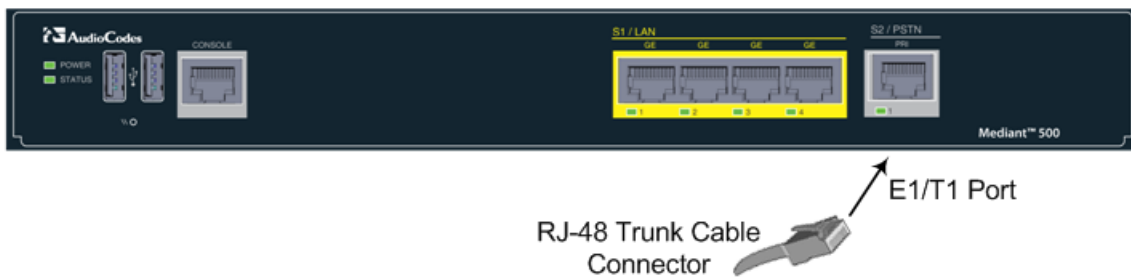
Figure 5-4: Cabling E1/T1 Port
