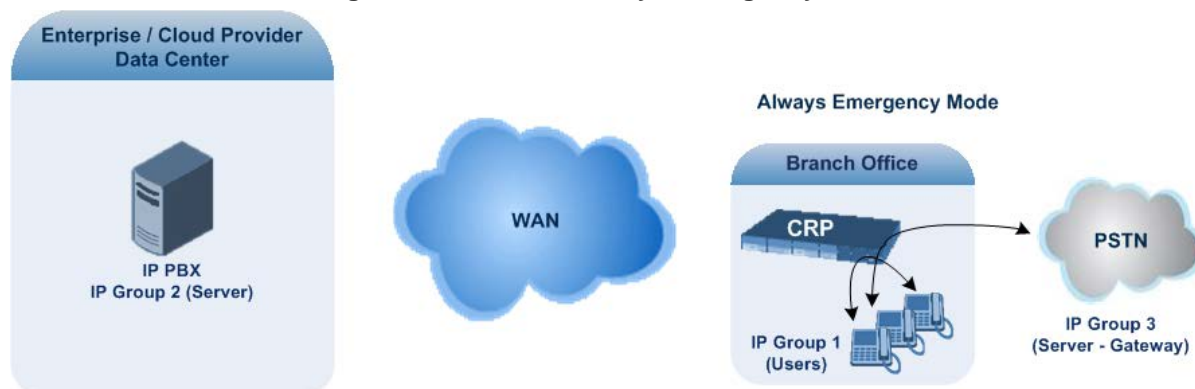
Figure 23-2: CRP in Always Emergency Mode
