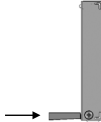
Figure 6-3: Module Handle Pushed In (Top View)
