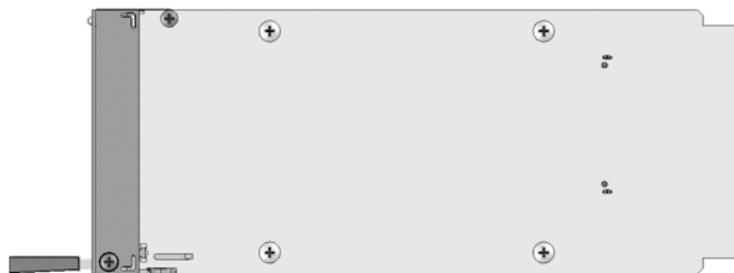
Figure 6-4: Extracted Blank AMC Module (Top View)
