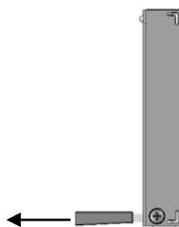
Figure 6-2: Module Handle Partially Pulled Out (Top View)
