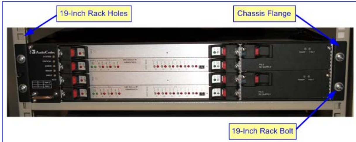
Figure 4-1: Chassis Mounted in 19-inch Rack
