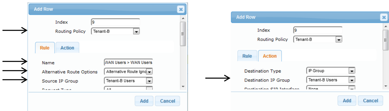
Figure 7-42: Alternative Routing Rule – Call Survivability of WAN Nomadic Users for Tenant B
