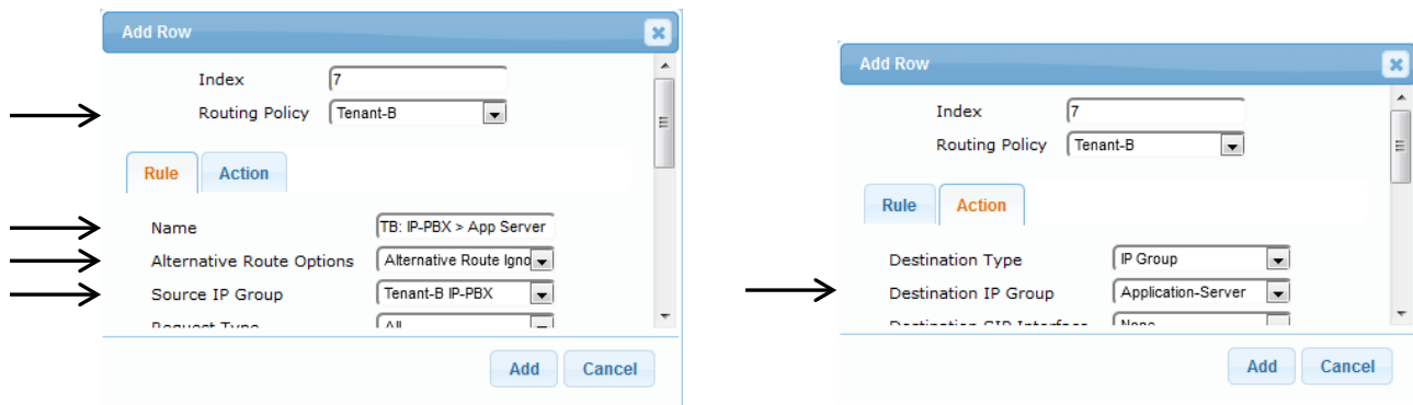
Figure 7-40: Alternative Routing Rule - HQ IP PBX to Application Server for Tenant B
