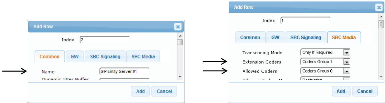
Figure 6-18: IP Profile for SIP Entity Server #1
