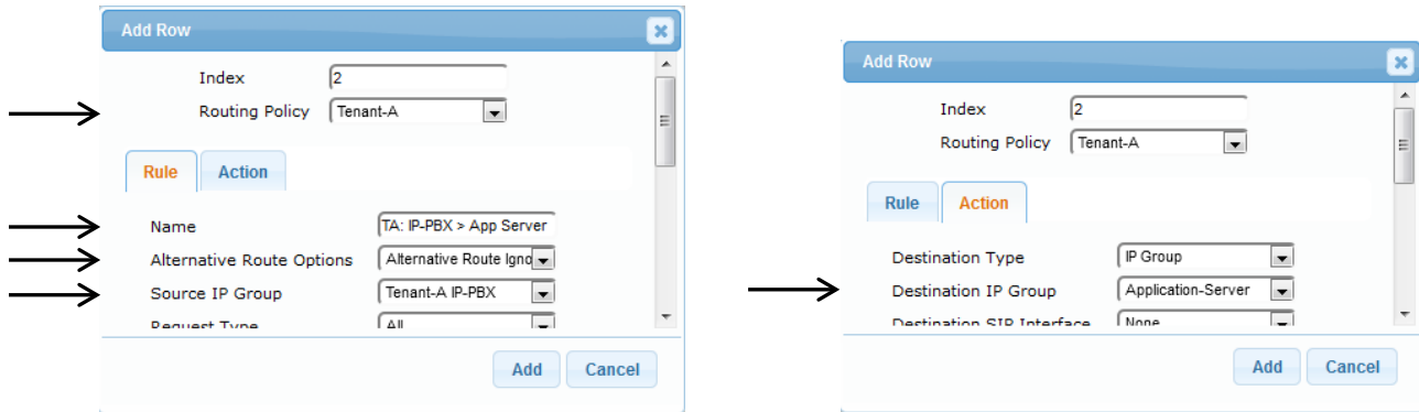
Figure 7-35: Alternative Routing Rule - HQ IP PBX to Application Server for Tenant A
