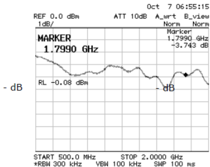
Insertion Loss Measurement
