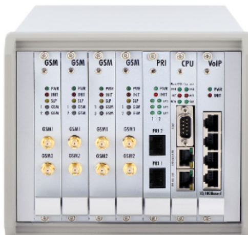
Figure: 2N® BlueTower with 4 UMTS Boards, Basic CPU, 2 ISDN PRI, VoIP Interfaces
