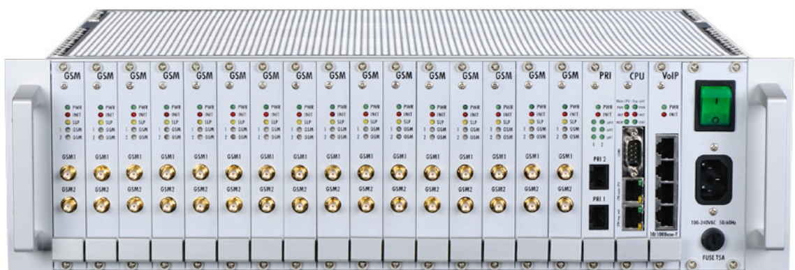
Figure: 2N® StarGate with 16 UMTS Boards, Enhanced CPU, 2 ISDN PRI, VoIP Interfaces and AC Power Supply
